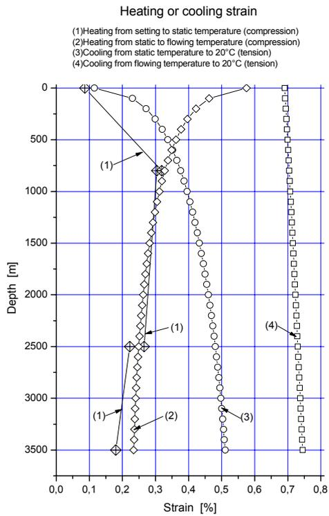
**Figure 7: One-dimensional strain from hindered thermal expansion.**
