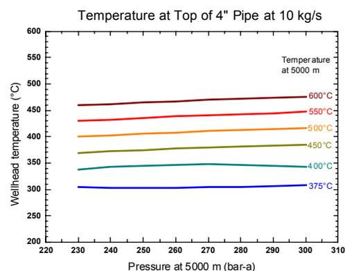
Figure 2. Wellhead temperature.
