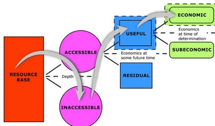
**Figure 1: A slightly modified McKelvey diagram. The arrows are meant to indicate that the IDDP deep drilling could result in an increase of the *accessible* portion of the *resource base* at the expense of the *inaccessible* portion. And an increase in the *useful* and *economic* portions as well (also indicated by the dotted frames around the two boxes).**
