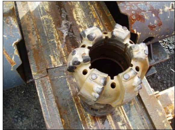
Figure 7: A close-up picture of Baker Hughes PDC core-bit after the 1st spot coring operation in well RN-19. Some of the PCD's were chopped and one was damaged
