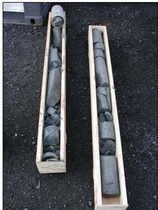
Figure 8: The core cut into a dolerite intrusion with high angle actinolite veins that are quite visible in the box to the left. The top of the core is in the box to the right - bottom right corner of the image, looking downwards. The boxes are 1.6 m long and the aluminum liner is still around the bottom of the core
