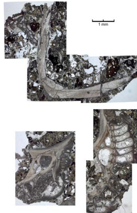
Figure 5: Microscopic images of shell fragments from 630 metres in well RN-10. The upper is probably a mollusk and the two lower barnacle fragments, which seem to be somewhat re-crystallized
