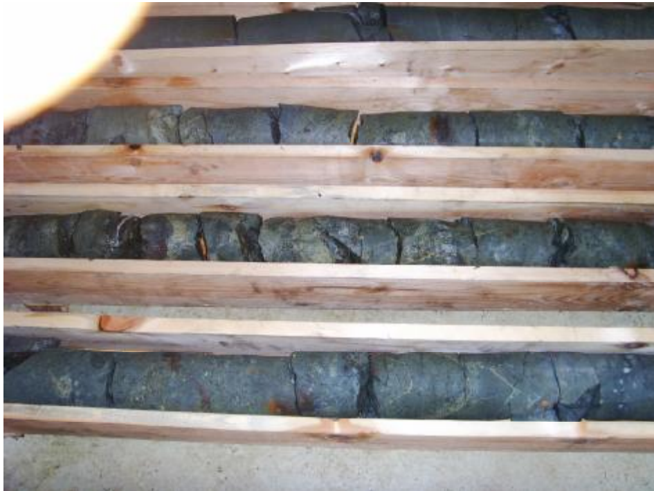
Figure 13. A close up of the core boxes containing green hyaloclastite breccia.
