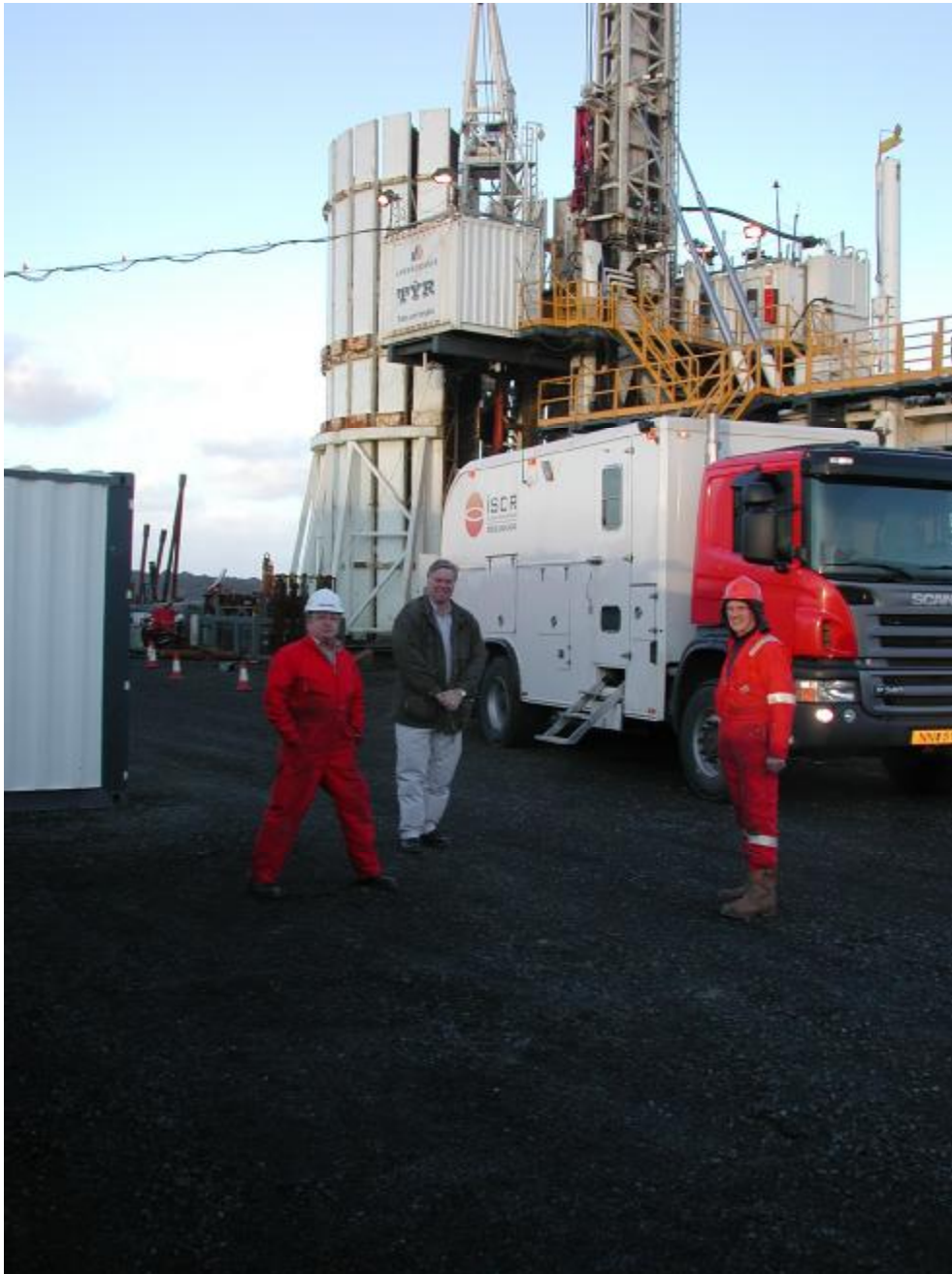
Figure 19. The drill rig Tyr is scheduled for the IDDP-1 well in Krafla in March 2009 – and will begin by drilling a 17 ½" well from 800 m to about 2400 m depth, followed by inserting and cementing of the 13 3/8" casing. Then a 12 ¼" drilling to 3500 m – including several spot cores, and casing by 9 5/8" cemented casing. The well will be completed by 8 ½" rotary drilling to 4500 m depth, including several spot cores.
