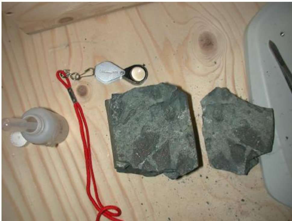
Figure 14. Preliminary inspection of the drill core. The core contains base metal sulphides, epidote, actinolite and quartz in abundance, but no calcite (suggesting T > 300^{\circ}\text{C} ).
