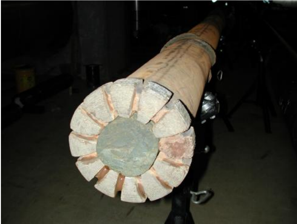
Figure 11. The core was out of the hole some 11 hours after coring. One tooth damaged – otherwise a healthy bit and a core inside the barrel.
