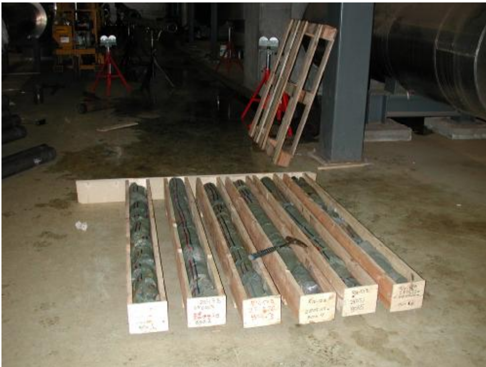
Figure 12. 6 boxes, 1.65 m each, full of 4" drill core.
