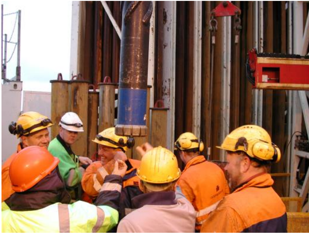
Figure 7. Core barrel on its way down to the drill hole.
