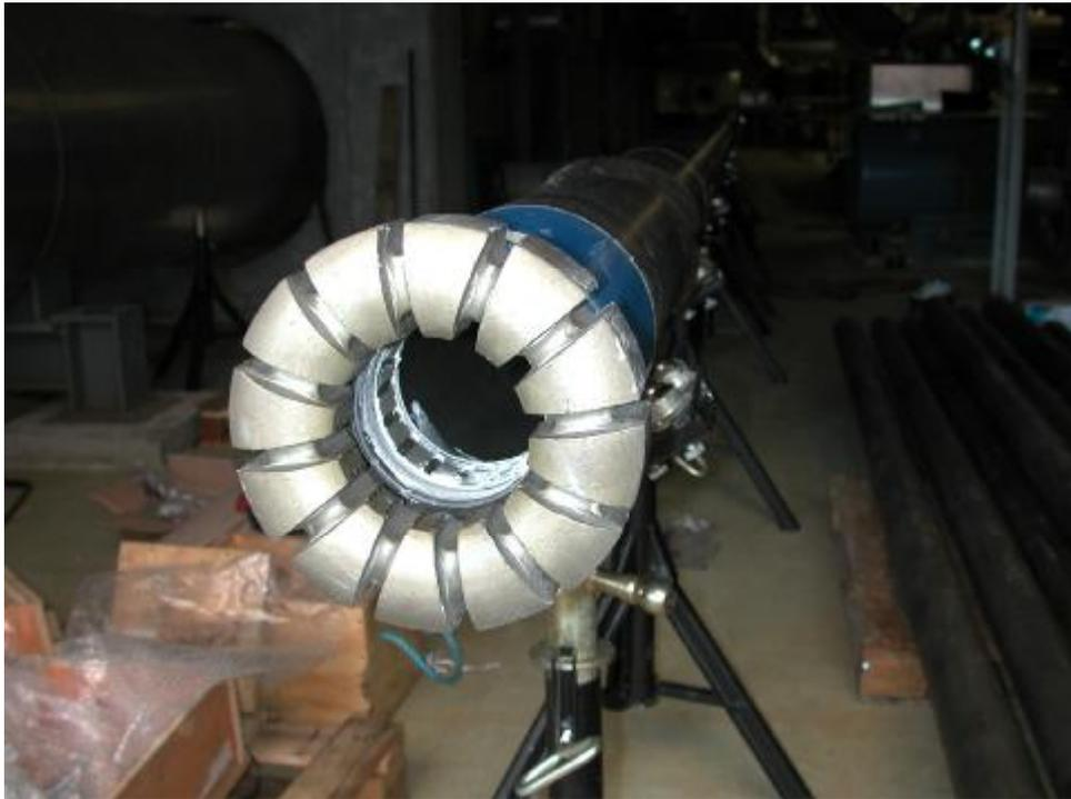
Figure 5. The core bit and the core catcher.
