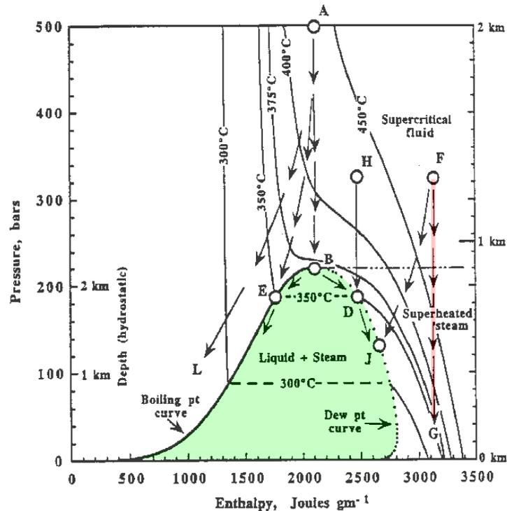
**Figure 4:** Pressure enthalpy diagram for pure H<sub>2</sub>O with selected isotherms. The conditions under which steam and water coexist is shown by the shaded area, bounded by the boiling point curve to the left and the dew point curve to the right. The arrows show different possible cooling paths (from Fournier, 1999).
