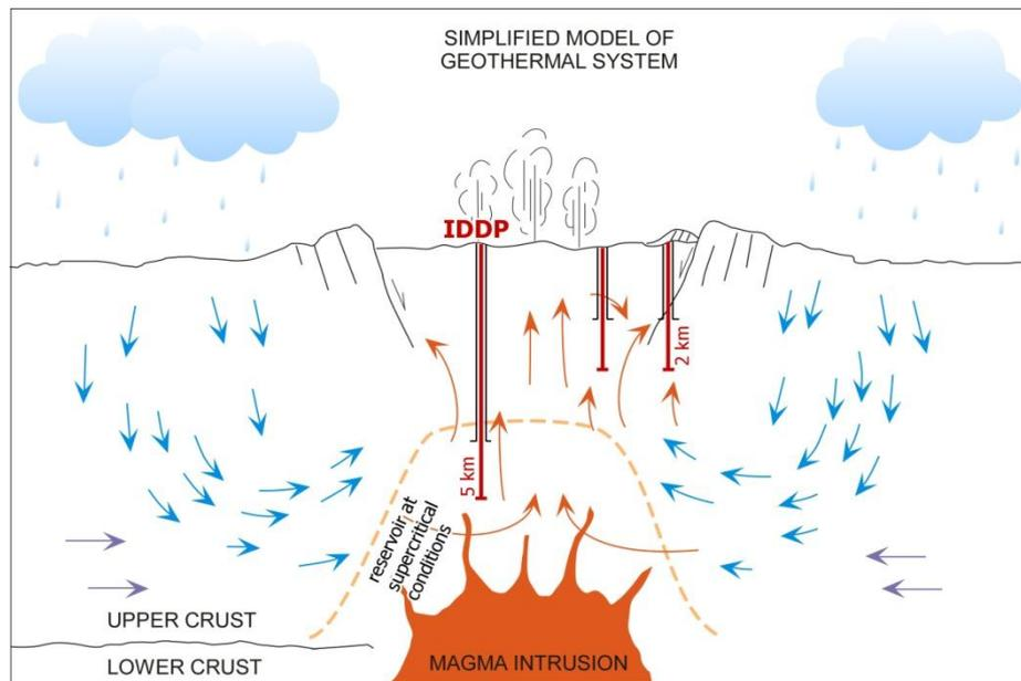
**Figure 5.** A simplified geothermal model showing schematically a reservoir at supercritical conditions surrounding a magmatic heat source. It is of vital importance that the IDDP production casing reaches down into the supercritical reservoir.
