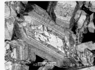
Figure 1. Back scattered electron photomicrograph showing complex oscillatory zoned epidote with Fe-rich cores and Al-rich rims from 1430 m depth in well RN-10 at Reykjanes.
