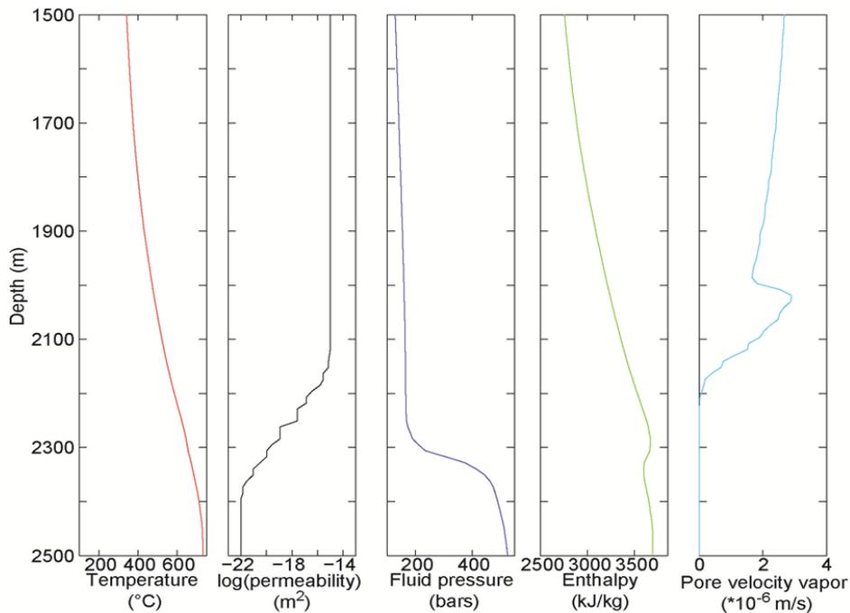
Figure 3. Changes in temperature, permeability, fluid pressure, enthalpy and pore velocity vapor in the zone of superheated steam above the intrusion, along the black line shown in Figure 2.
